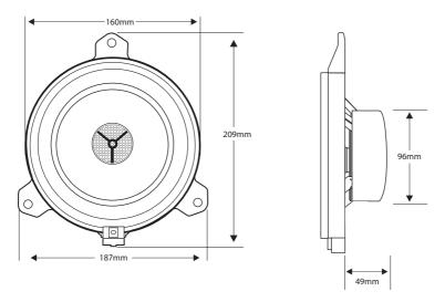
Pair of 6.5" Toyota plug & play 2-way coaxial speaker to upgrade OE speaker for selected models with Polypropylene Cone including mounting hardware
